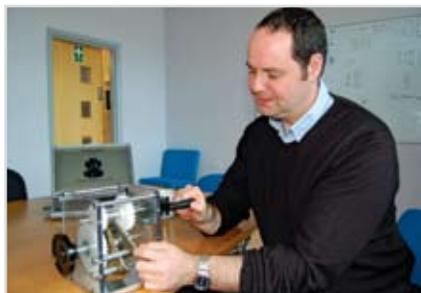
**Because it uses a conventional gear linkage and fits into a regular transmission case, the Zeroshift seamless-shifting technology could be easily and inexpensively adapted to existing engine designs.**
