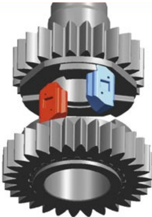
Figure 5: Second gear engages with the bullet accelerating the ZeroShift hub
