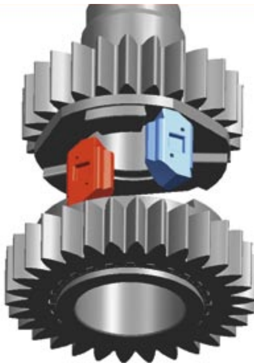
Figure 6: Second gear overdrives first gear unloading the first gear bullet (blue)
