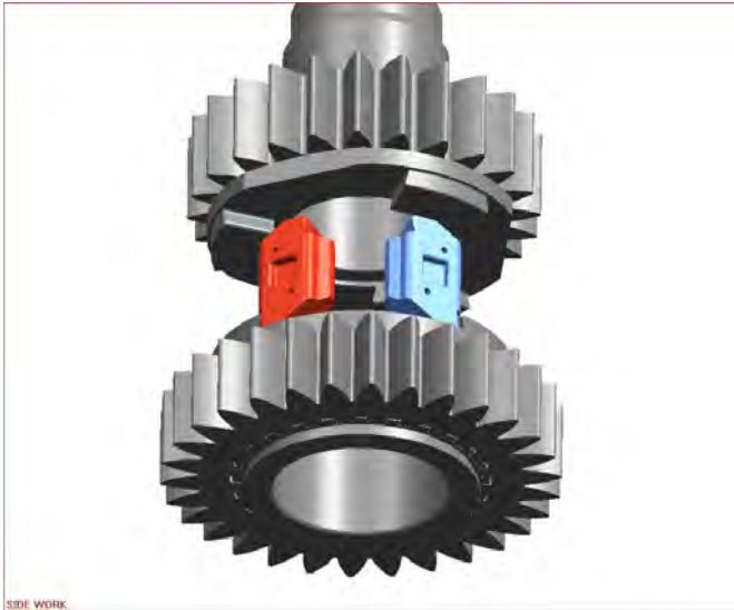
Figure 6. 2 nd gear engaged.
