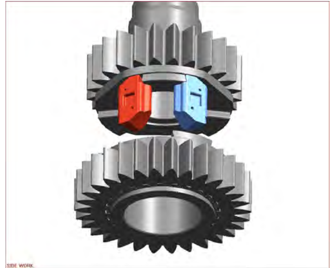
Figure 4. 1 st gear engaged.
