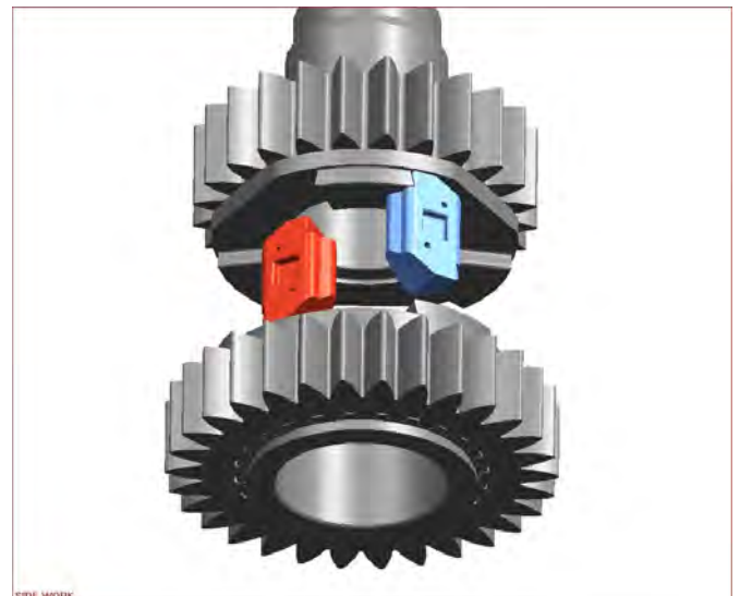
Figure 5. 2 nd gear overruns 1 st gear.
