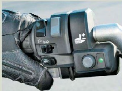
Yamaha's FJR1300A uses an electronic clutch to shift gears
